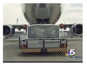
One of the planes was in the air, and the other was being pulled on the ground by a special tug bought by American to save fuel.
